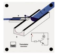
... reaches the base, this flow of water opens the slide and makes the way free for the large water flow (collector emitter line), the water can flow.
