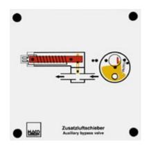
If the engine speed is too low, the cross-section is reduced, the output rotor turns more quickly.
