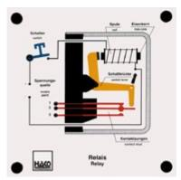
... the contacts of electric circuit 2-1 over to circuit 2-3.
